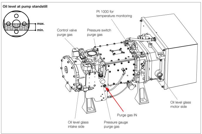
Fig. 3.2 Connections and controls
