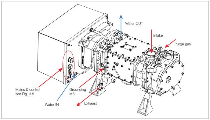
Fig. 3.1 Connections to the DRYVAC DV 200/300/500
