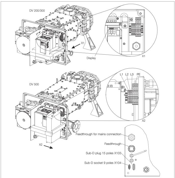
Fig. 3.5 Frequency converter without covers
