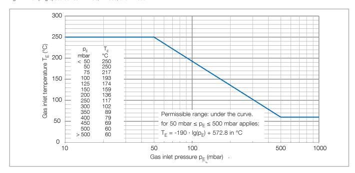
Fig. 1.2 Permissible gas inlet temperature as function of the inlet pressure
