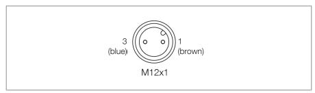
Fig. 3.7 Purge gas pressure switch connection
