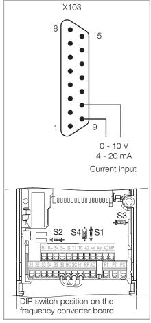
Fig. 4.5 Changing the speed of the pump
