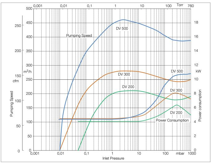
Fig. 1.1 Pumping speed curves DV 200, DV 300, and DV 500
