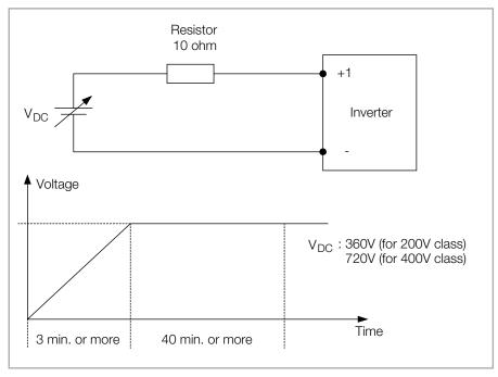
Fig. 2.2 Capacitor forming
