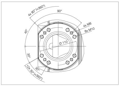
Fig. 3.3 Intake flange
