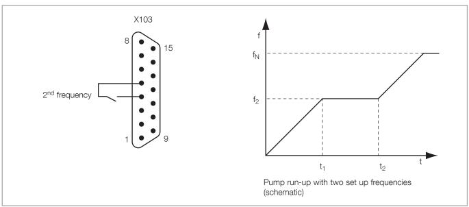
Fig. 4.4 Changing the speed of the pump
