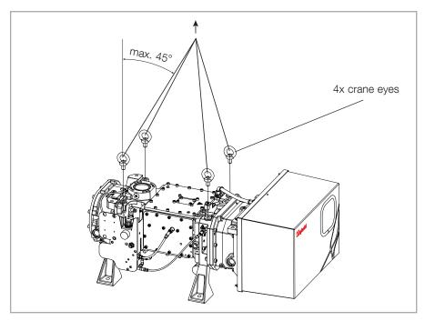
Fig. 2.1 Lifting the DRYVAC
