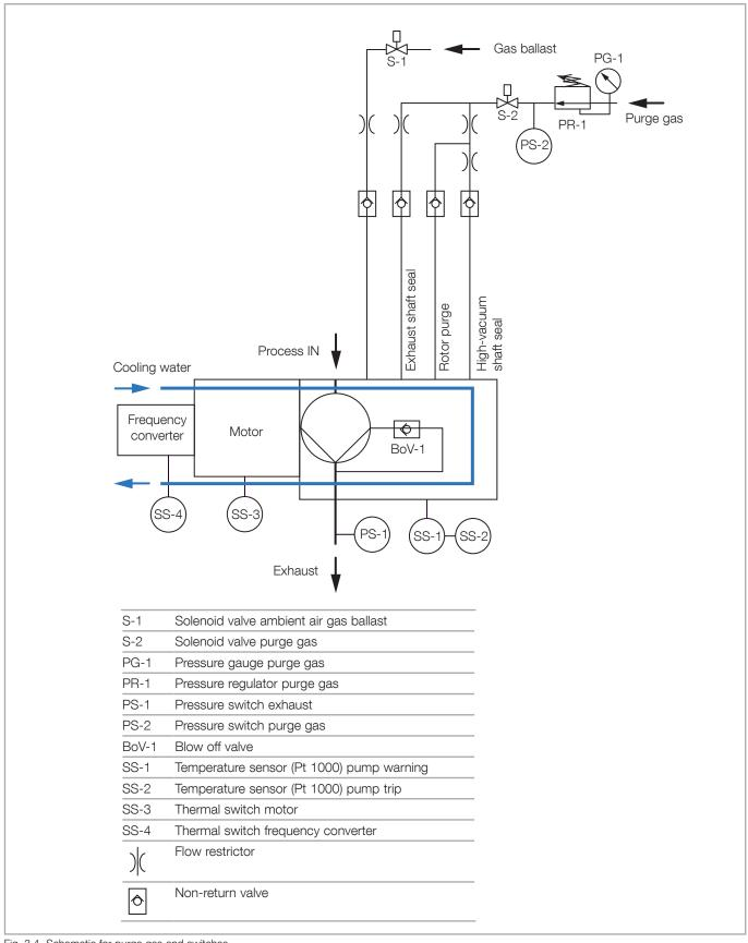
Fig. 3.4 Schematic for purge gas and switches
