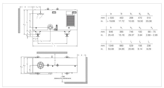
Dimensional drawing for the SCREWLINE SP 250
