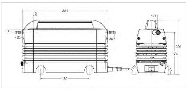
Dimensional drawing for the DIVAC 1.4 HV3C
