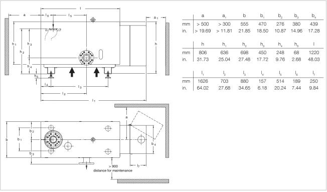
Dimensional drawing for the SCREWLINE SP 630
