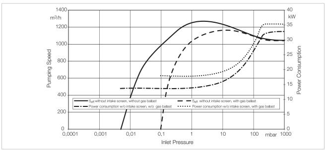
Pumping speed curves of the DRYVAC DV 1200 and DV 1200 S-i
