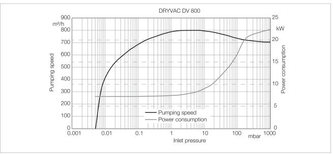
Pumping speed curve of the DRYVAC DV 800
