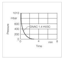
Curves of pump-down time of a 10 I vessel
