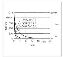
Curves of pump-down time of a 10 I vessel
