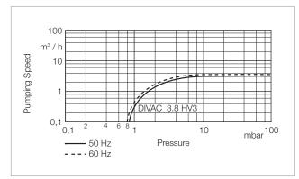
Pumping speed curve of the DIVAC 3.8 HV3
