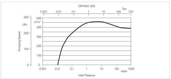
Pumping speed curve of the DRYVAC DV 500
