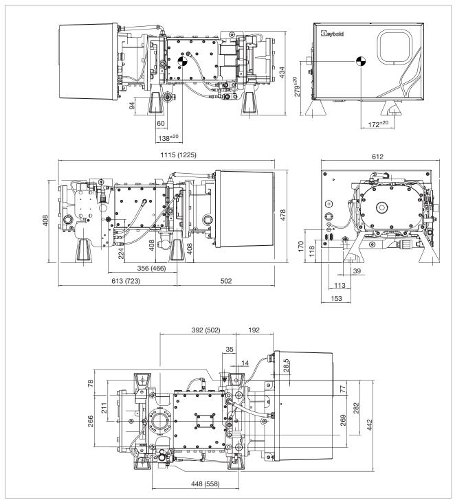
Dimensional drawing for the DRYVAC DV 200, DV300 and (DV 500), all dimensions in mm
