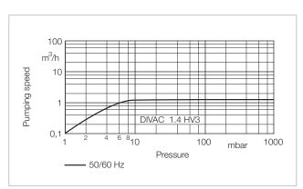
Pumping speed curve of the DIVAC 1.4 HV3
