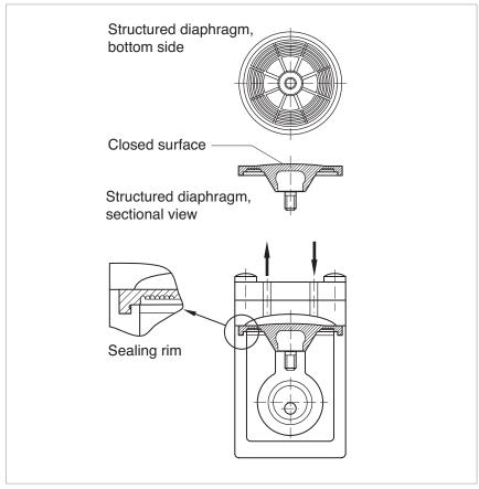
The structured diaphragm with its sealed surface provides the basis for a long service life and a low base pressure.
